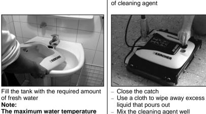
The maximum water temperature must be 50°C.
